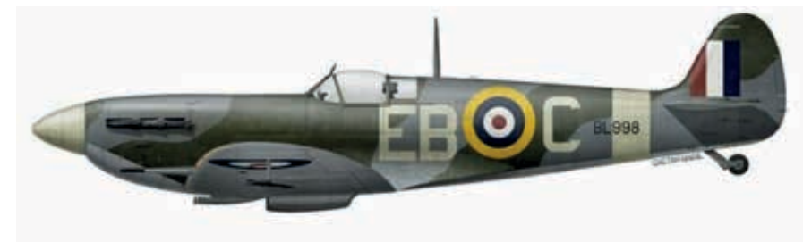
Supermarine Spitfire EB-C as flown by Sgt Goodall. Armed with two Hispano 20 mm canons and four Browning.303 machine guns it could also carry two 250 lb or one 500 lb bombs. Powered by a Rolls Royce 45 series V12 engine that developed 1,440 HP
